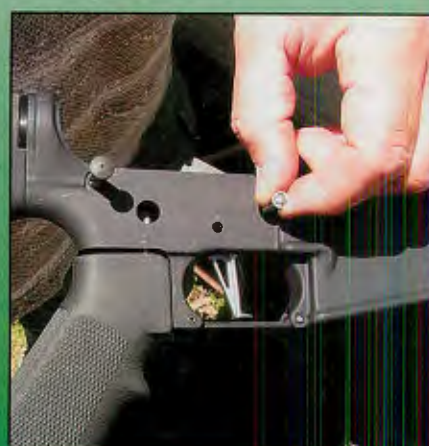
Secure Super Match Trigger Group by inserting new retaining pins with punch or drift. E-clips secure retaining pins.
