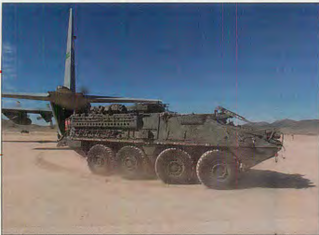
Lead elements of Stryker Brigade deploy in the desert. The eight-wheeled vehicles have been criticized as too heavy to deploy by air, and prone to sinking into soft sand and mud.
