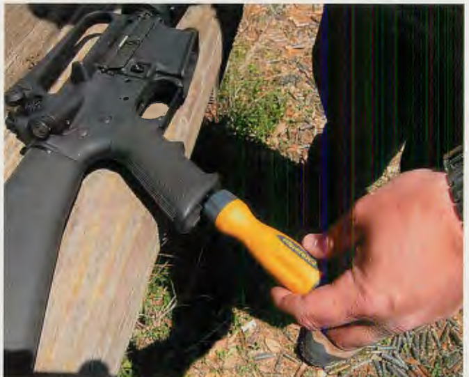
Use screwdriver or hex wrench to loosen pistol grip.
