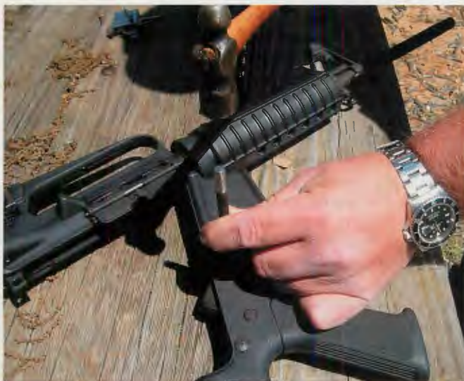
Installation starts by using a punch or drift to drive trigger-group retaining pins from AR-15 receiver.
