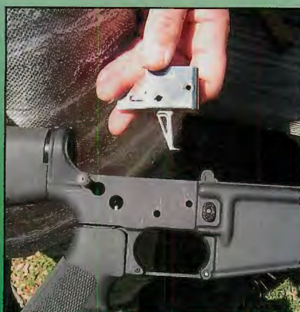
Insert Super Match Trigger Group into trigger-group pocket.
